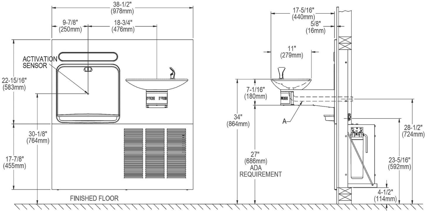
NOTE : New Installations Must Use Ground Fault Circuit Interrupter (GFCI). It is highly recommended that the circuit be dedicated and the load protection be sized for 20 amps.
